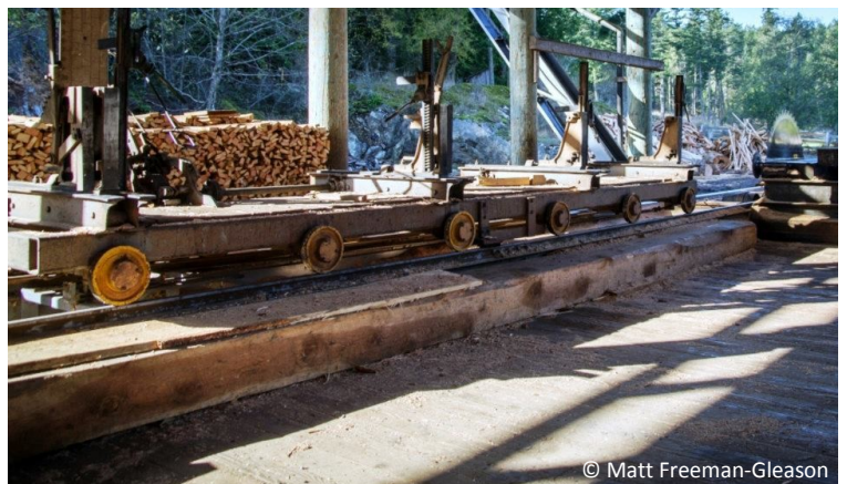
This log carriage runs logs through the circular saw in the top right of the picture. The equipment is capable of milling large diameter logs.
