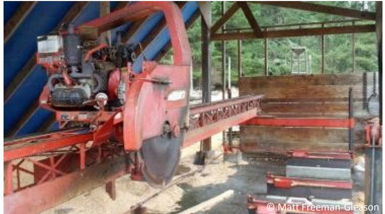
Bond Lumber Mill's Mobile Dimension circular saw can break down small and large logs.
